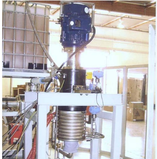
A commercial size STT ® reactor capable of producing over 13 million gallons per year of biodiesel from various feedstocks.
